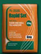
Rapid Set is a rapid setting cement based floor and wall tile adhesive with improved slip resistance. Rapid Set has been developed for fixing porous tiles such as ceramic, quarry and terracotta tiles to solid substrates such as sand/cement screed and concrete. Its rapid setting capability allows for light foot traffic and grouting after 3 hours. Rapid Set can be used internally and externally and it is unaffected by frost after setting.
