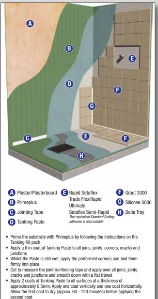
Tiling can commence once the Tanking Paste has dried, usually 3 – 4 hours depending on the substrate and the application thickness
