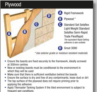
Max tiling weight (dependant on board type & thickness) is 30kg/m<sup>2</sup> inc tiles, adhesive & grout
